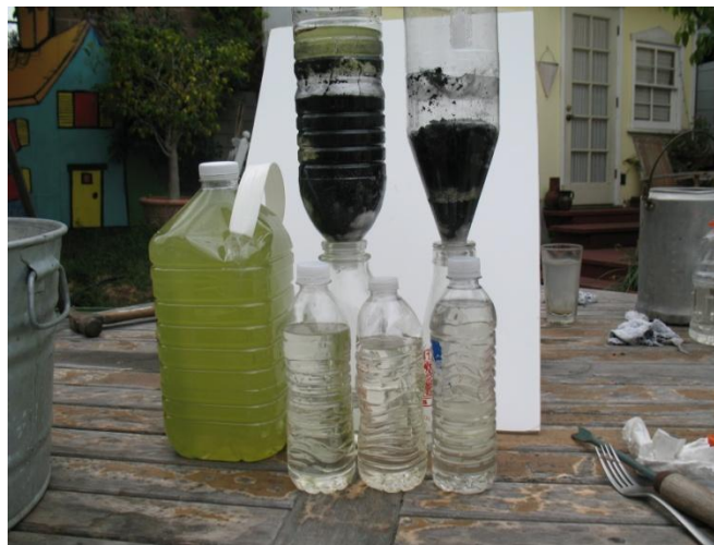
Figure 4 Untreated Greenish Water On The Left, Filtration In Process On The Right
